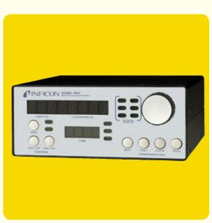
The TF-SQM160 uses proven INFICON quartz crystal sensor technology to measure rate and thickness in thin film deposition processes. Two sensor inputs are standard and four additional sensor inputs are optional. Two recorder outputs provide analogue rate and thickness signals.
