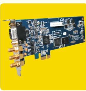
The TF-IQM-233 PCI Express card turns your PC into a thin film deposition controller. This INFICON designed and manufactured product is the ideal choice for system OEMs, or anyone wishing to incorporate a thin film deposition controller into an existing PC or PLC controlled system. Installation is simple—all you need is an unoccupied PCI Express slot. TF-IQM-233 is available to fit in standard or small form factor PC towers.
